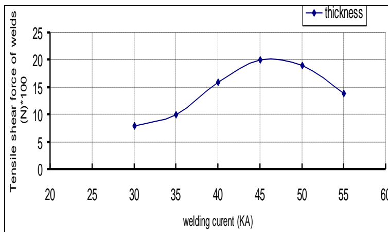
Fig(7):- Effect of welding current (KA) on weld quality at constant electrode pressure and thickness ( p=1.5 KN& t=1.5 mm)
