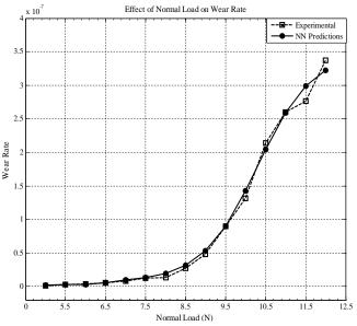
**Fig.(7):**Comparison plot for predicted and experimental values at constant Speed (1.5m/s) and Time (2hr).
