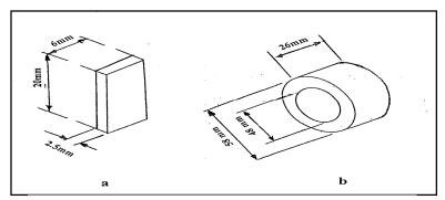
**Fig.(1):** A specimen a) Pin b) Tested ring
