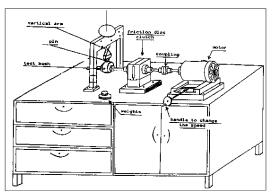
Fig.(2): Wear Test Machine .
