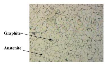
Fig.(9): Microstructure of welding zone (Mag. X65).
