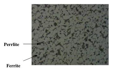
Fig.(8): Microstructure of nudulare cast steel (Mag. X130).
