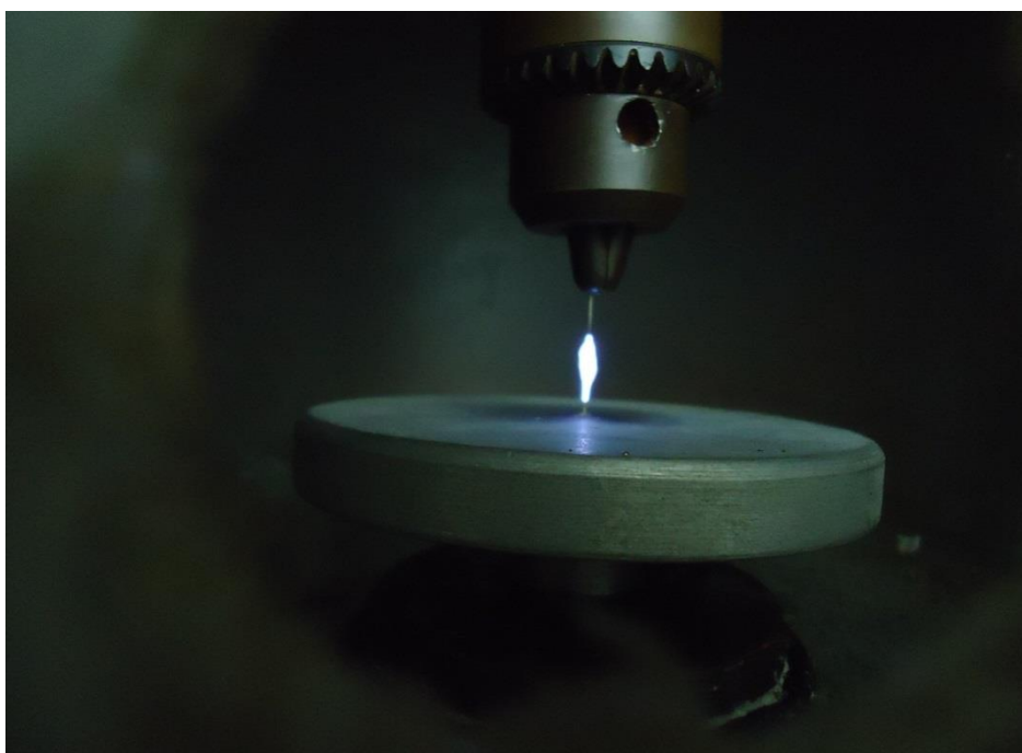
Figure (13): Photograph represent the corona and breakdown voltages in pin to pin Electrode geometry.
