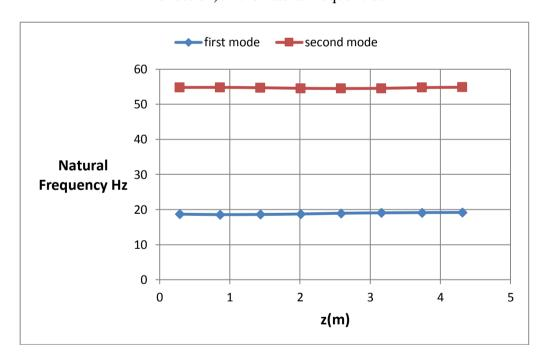
Figure(9) The effect of the damage panel location along the wing span (z-direction)on the natural frequencies.
