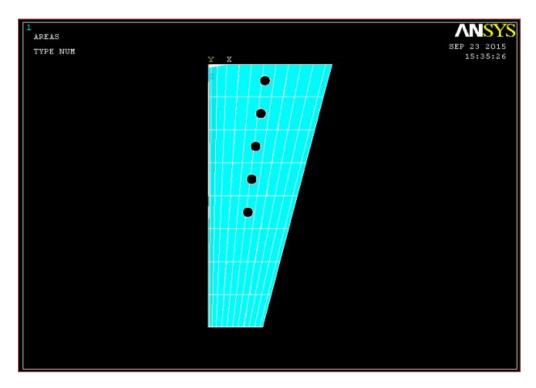
(c) Cutout at the center of five panels along the wing span with cutout ratio=0.2. Figure (4) Cutout in a different panels locations and different cutouts ratios.
