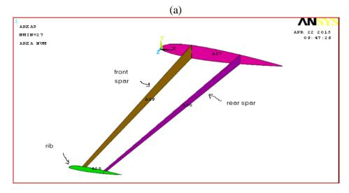
(b) Figure (1) The wing model used in the Analysis
