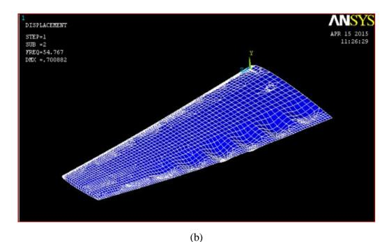
Figure (5) Natural mode shapes when the cutout at the center of the root panel between front and rear spar at (d/D)=0.2. (a) first mode (b) second mode.
