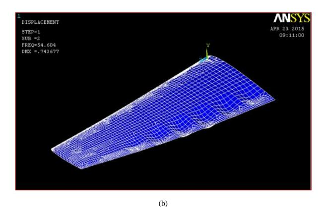
Figure (6) Natural mode shapes when the cutout at the center of the tip panel between front and rear spar at (d/D)=0.2. (a) first mode (b) second mode.
