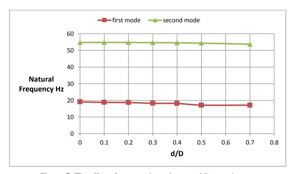
Figure (7) The effect of cutout ratio on the natural frequencies.
