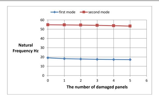
Figure(10)The effect of the number of damaged panels on the natural frequencies.
