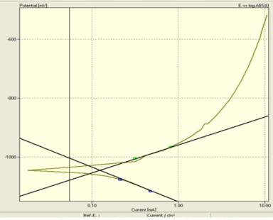
Fig. 2: Polarization curves of galvanized Electrical Bar Stands (thickness 120  $\mu m$ ) in 3.5% NaCl
