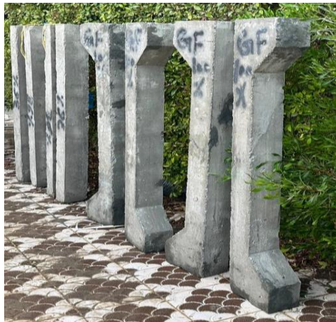
Figure 4. R.C. columns specimens
