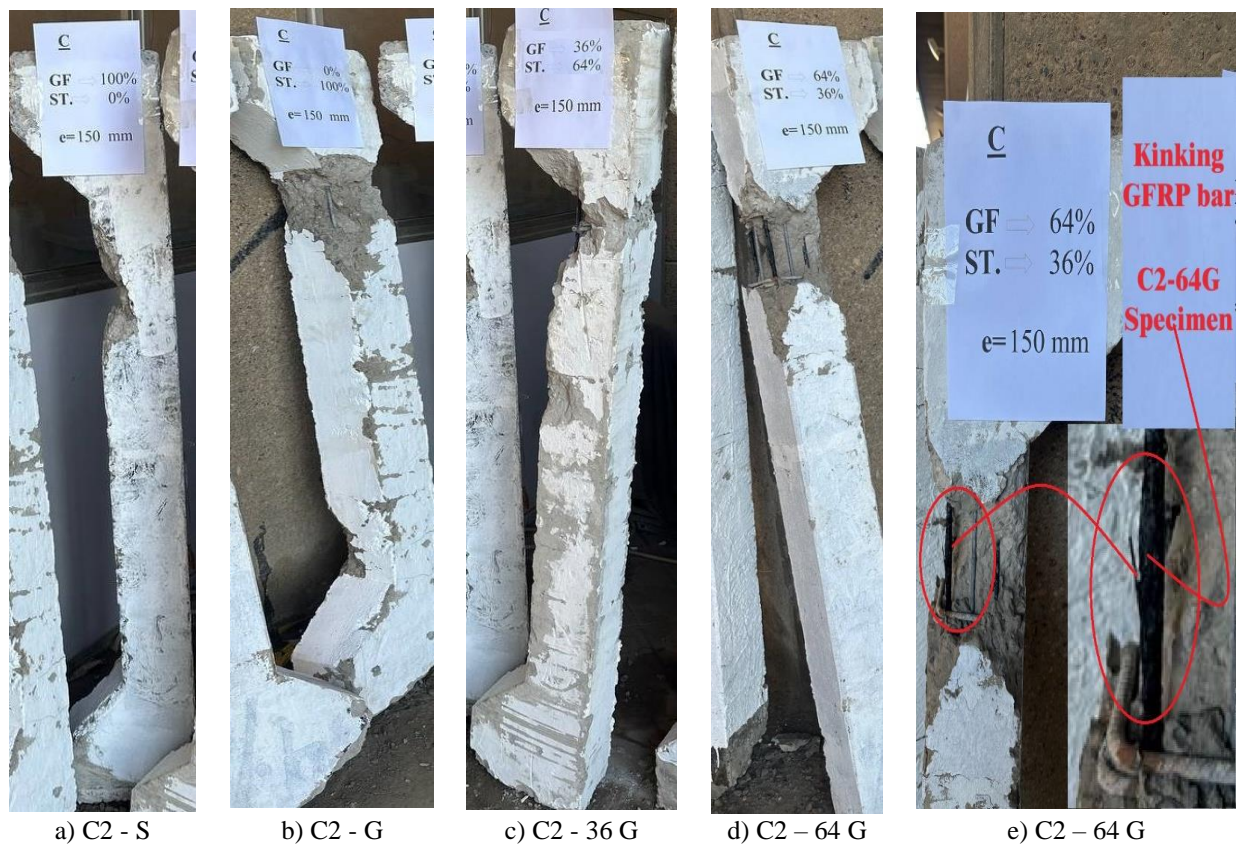
Figure 10. Failure modes for R. C. columns specimens with eccentricity ratio e/h=1
