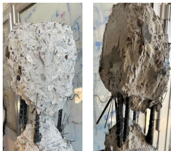
Figure 8. Kinking in GFRP bars that occur in the compression zone for the specimens [N-G]
