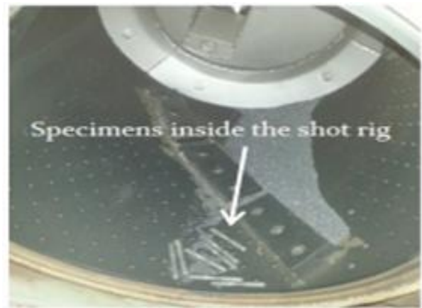
b. (SP) treatment with samples inside the container rotation
